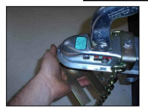
Insert dummy ring plate when trailer is unhitched by lifting handle and pushing into place.
