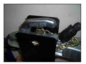
**3.** Offer up bottom channel with the tall fill in strip at the front. Ensure the chain does not infringe on the hole as it will prove difficult to insert the lockbar.
