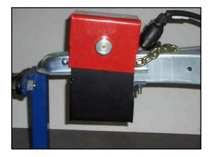
Place the red top box over the bottom channel and lower until holes line up.
