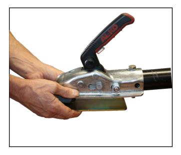
When the trailer is unhitched lift the handle to insert the dummy ring plate, until it clicks into position and releases the handle.
