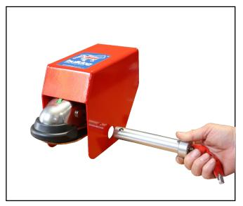
Insert the lock bolt through both holes of the cover. Fit the recessed cup over the end of the lock bolt, then turn the key a quarter turn clockwise to lock and remove key.
