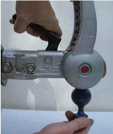
2. With the stabiliser handle in the upright position, lift the hitch handle and insert the dummy ball.
