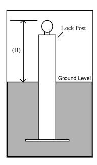
2. Concrete post in while ensuring that it remains in a true vertical position with the aid of a spirit level.
