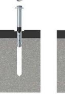
Line up the safe and insert the bolt. Tap the bolt in with a hammer.
