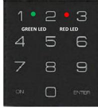
A short buzzer note and green LED light validate every keypad entry (except the "ENTER" key). If more than 10 seconds elapses between button entries or if the complete code entry exceeds 30 seconds in length the lock will automatically go back into "sleep mode" and the code entry process needs to begin again.
