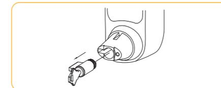
3. To replace cylinder, reinsert and turn 90° clockwise. Replace the cylinder cover and handle.
