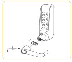
2. Turn Kev 90° anticlockwise and remove the cylinder from boss.
