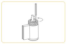
5. Refit the tailpiece, hold down the control pin and screw the cap on fully without tightening. Ensure the control pin projects to lock the cap.
