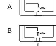
Step 2. Fasten the anchoring device to the floor using the included screws.
