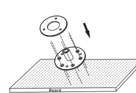
Step 3. Place the safe down over top of the anchor and fasten with the Allen bolt.
