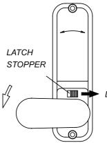
If your door is left hand, turn the handle 90 degrees to the left and slide the latch stopper to keep up the handle The hold open function is now working.
