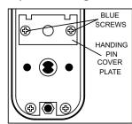
The Exterior Code Pad Assembly is usually factory set for left hand door handing. (The outer knob will turn freely in an anticlockwise direction and resist clockwise turning).
