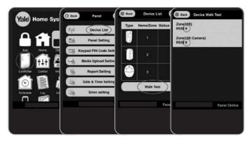
Hold the devices in the desired location and press the Test/ Learn button (see below) on the accessories.
